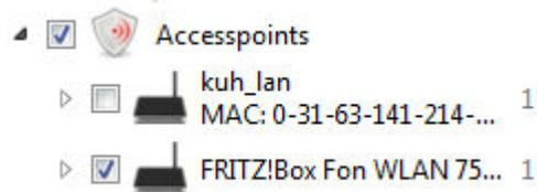
*signal strength:* all accesspoint are used by the WLAN scanner but only for the strongest signal a measurement is calculated and a measure point is set.
