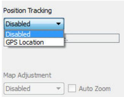
If a GPS device is connected it should take 5 – 20 seconds until the first valid position is detected. In that case the position is displayed within the *Position Tracking* window.
